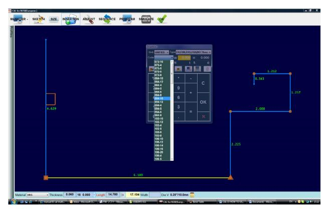
Click type to choose pull down menu from library Click code from pull down menu Enter the distance from start or end Enter number of fasteners Enter the space between fasteners
